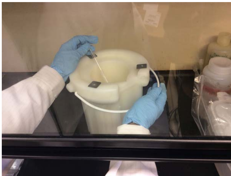
Figure 4: Showing Dewar flask containing dry ice and acetone used for instant freezing
