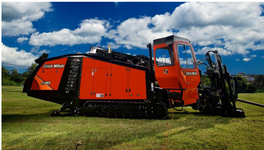
Figure 8: This type of drill rig is used for utility line installation (Ditch Witch, 2015).
