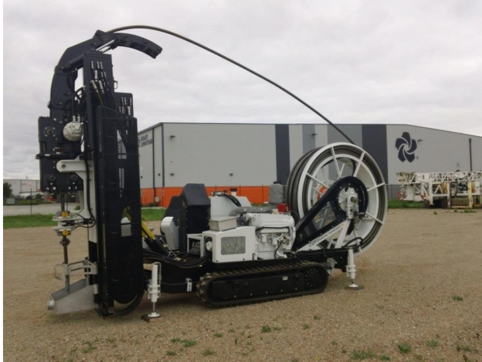
Figure 9: The prototype developed by the DET CRC. This drill rig utilizes the coil tube technology for mineral exploration (Probert, 2013).
