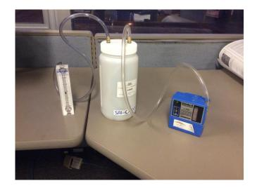
Figure 1: Sampling pump calibration
