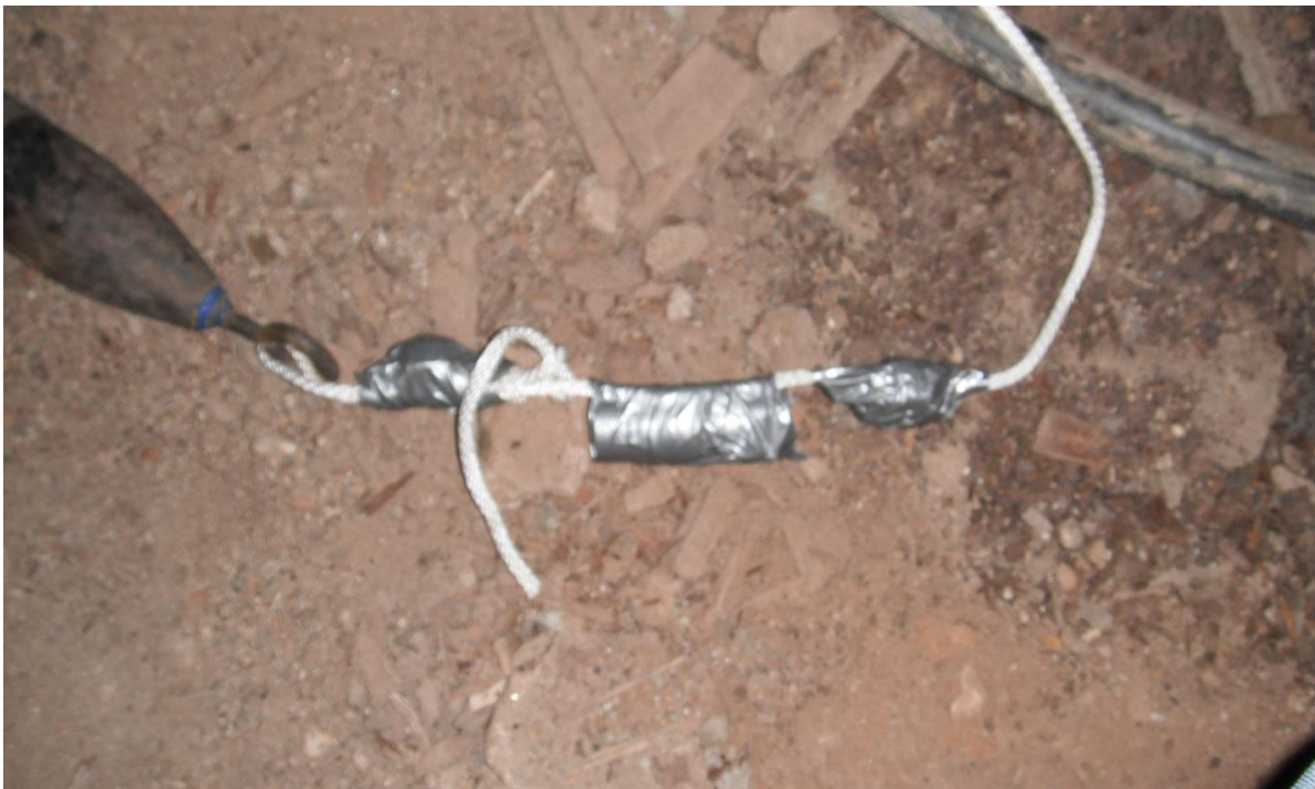
Figure 5. Pictured here (from left to right) is: one 20 kg slug, one Hobo Tidbit temperature logger, one Star-Oddi Seastar DST CTD miniature salinity/temperature/depth logger, another Hobo Tidbit, and 3/8" nylon rope.
