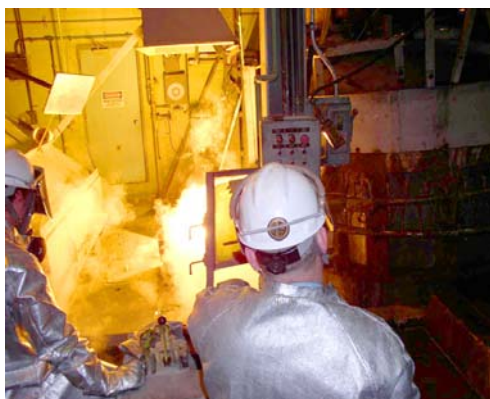
Figure 3. Pouring Molten Beryl Frit - Be Extraction
