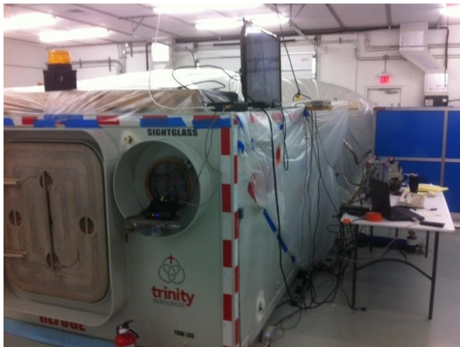
Figure 8: Trinity Resources 10 person mine refuge alternative modified with CryoRASS system (Doerr D. , 2013)
