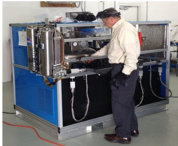
Figure 11: Cryogenic Air Servicing and Fill Station (CryoASFS) filling a CryoBA pack (Doerr et al, 2013)
