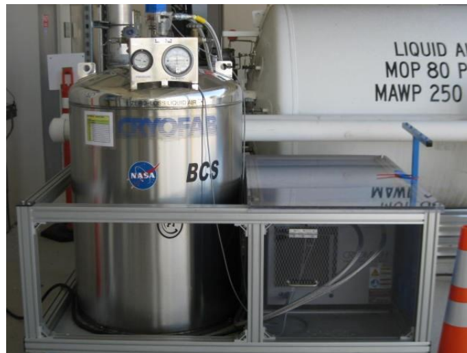
Figure 12: Zero Loss Dewar prototype (Goetzfried & Madgett, 2012)
