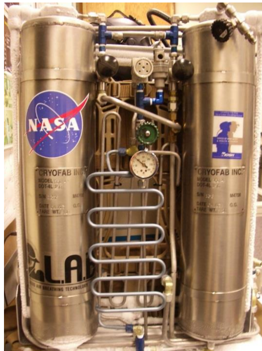
Figure 10: Cryogenic Breathing Apparatus (CryoBA) pack (Doerr et al, 2013)
