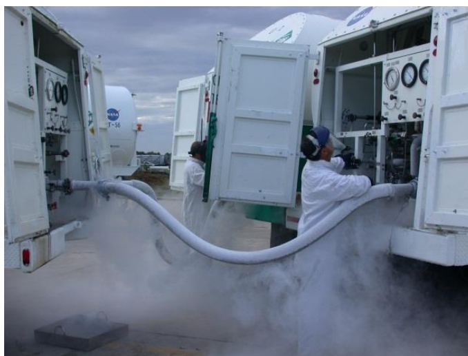
Figure 13: The production of liquid breathing air from liquid oxygen and liquid nitrogen tankers (Doerr et al, 2013)
