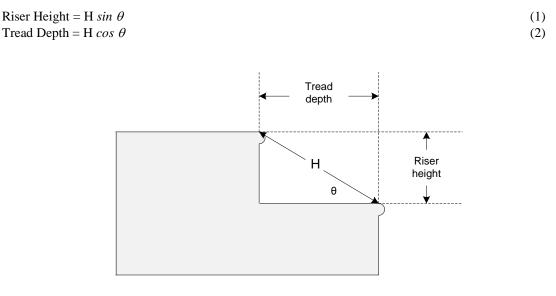
Figure 1. Step dimensions and angle used with the nosing-to-nosing measurement system.
