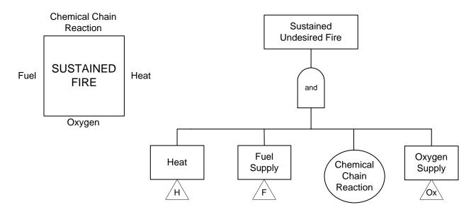
Figure 2. Fire Rectangle (left) and Corresponding Fault Tree (right)
