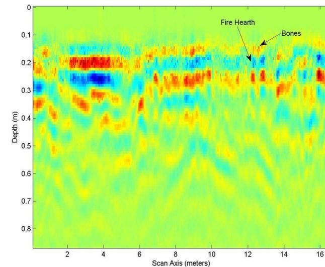
Left, a processed profile of GPR data. A depth conversion was performed using a calculated half-space velocity of 0.057 m/ns. The fire hearth is distinguishable by a strong contrast between its surroundings. Based on excavation results, accumulation of artifacts appears as narrowly-spaced groupings of steeply dipping diffraction curves.
