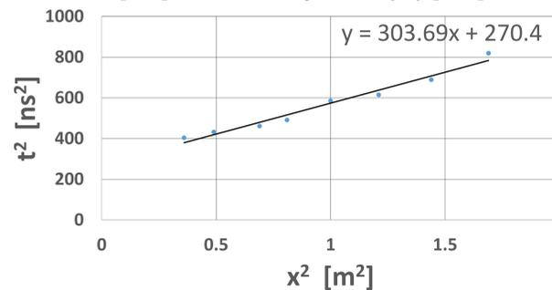
Left, a graph of the square of the antenna separation versus the square of the reflection traveltime from the common midpoint test. The square root of the inverse of the slope gives the half-space velocity which is used for depth conversion
