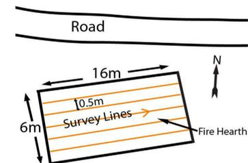
Left, a map of the survey grid. Along the width of the grid, stakes placed 0.5 m apart distinguish profile spacing. Along the length of the grid, GPR measurements were recorded every 0.05 m, utilizing unshielded 400 MHz antennas spaced 0.6 m apart.
