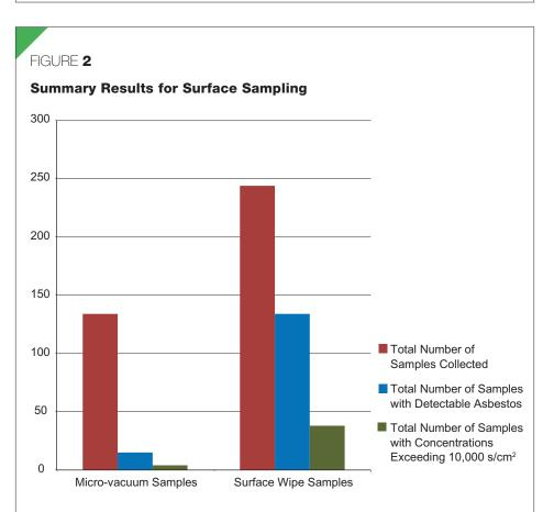
One hundred thirty-four micro-vacuum surface samples and 244 surface wipe samples were collected. Of these, 23 and 134 micro-vacuum and surface wipe samples, respectively, revealed detectable asbestos fibers. Four micro-vacuum and 38 surface wipe samples revealed asbestos concentrations exceeding the 10,000 s/cm<sup>2</sup> concentration adopted as the background surface concentration for our study.
