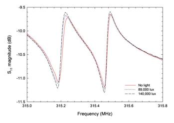
Fig. 9. (Color online) Different values of illuminance are measured using a single sensor tag loaded with a photodiode. Changing light intensity is indicated as a shift in the  $S_{11}$  magnitude and demonstrates sensor operation while affixed to the surface of a cylinder.
