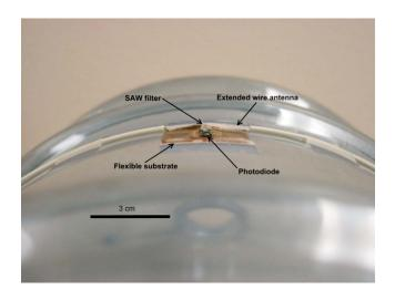
Fig. 8. (Color online) Sensor tag was fixed to the curved surface of a water container to test for functionality. The sensor was able to sense various levels of light while bent.
