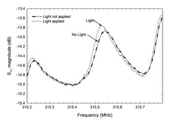
Fig. 7. (Color online) Measured  $S_{11}$  signals indicate an increased magnitude at the 315.50 MHz peak, representing illuminated conditions and decreased magnitude corresponding to decreased illumination.
