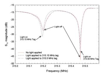
Fig. 10. (Color online) Incident  $S_{11}$  measurements at the network analyzer demonstrate that a pair of tags separated in operating frequency by 350 kHz is capable of individually sensing light vs dark conditions.
