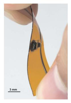
Fig. 3. (Color online) Prototype sensor tag made with 2.4 GHz components. The size of the resonant antenna scales inversely with frequency, allowing for a decrease in the antenna size over the 315 MHz SAW based sensor. Smaller components allow for even greater flexibility of the substrate.
