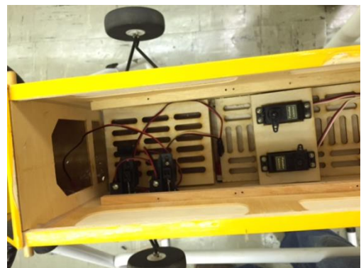
Figure 8 - Servo relocation and Battery Switches
