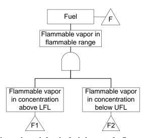
Exhibit 2. Fault tree branch for the fuel element of a flammable vapor fire.
