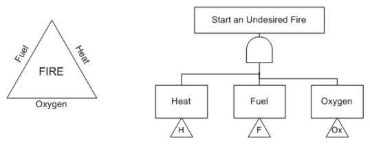
Exhibit 1. The fire triangle (left) and corresponding fault tree (right)
