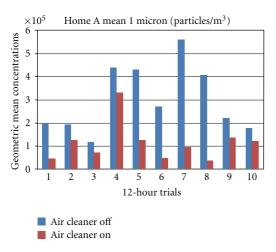
FIGURE 2: Geometric mean particle count concentrations (particle/ $m^3$ ) observed with the portable air purifier off and on at the one -m cutpoint for each 12-hour trial conducted in home A. Concentrations recorded with the air purifier on were consistently lower than concentrations recorded with the air purifier off. Similar observations were made in terms of particle concentration reductions with the air cleaner on at the other cutpoints.
